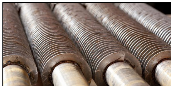
Surface area of spiral solid finned tube
